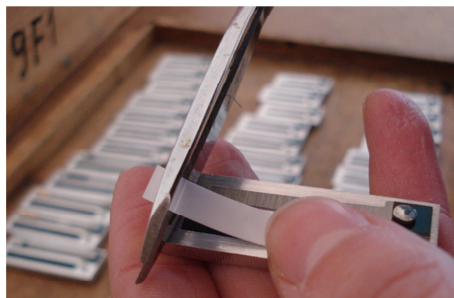
ASSEMBLAGE OF NATURAL/PLASTIC LEATHERS ON THE REEDS
