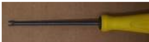
SPECIAL TOOL TO REGULATE POSITION OF THE KEYS
