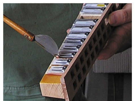
ASSEMBLY REEDS ON THE WOODEN REED-BLOCKS WITH WAX
