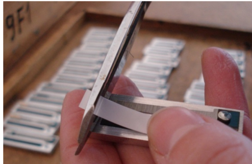
ASSEMBLY OF NATURA OR PLASTIC LEATHERS ON THE REEDS
