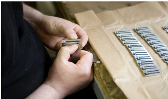
ADJUSTMENT OF THE TONGUES OF THE REEDS
