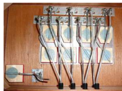
EXAMPLE OF A BASS MECHANISM IN A DIATONIC INSTRUMENT
