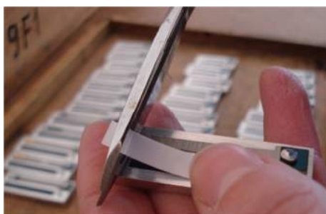
ASSEMBLAGE OF NATURAL/PLASTIC LEATHERS ON THE REEDS
