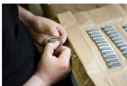
ADJUSTMENT OF THE TONGUES OF THE REEDS
